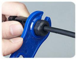
Use spanner to tighten the screw on both sides.
