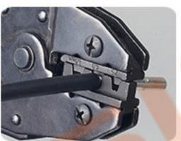
Put the stripped cable into the pin, crimp it tightly until loosen.
