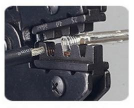
Put the metal pin to crimping tool tooth, and crimp lightly.
